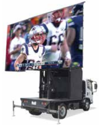
SuperMAX 17' x 10' screen 6mm pixel pitch 864 x 480p resolution
